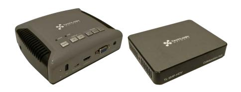
The TechLogix TL-SMP-HDV is an HDMI and VGA collaboration system which includes a control system to turn on and off the display and adjust the volume on the display with physical buttons on the top of the transmitter. The display may be controlled by CEC or IR commands. EDID information from the display is passed to the HDMI input, which supports video signals up to 4K/30. The VGA input can be configured to scale the source image up to 1920x1200.
