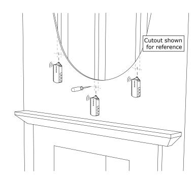
Cut out the opening along the Template tracing. Do not (13a) cut deeper than needed to cut the wall covering, there may be components of the fireplace behind the wall that could be damaged.
