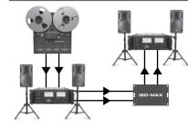
Using two amps in series Some installations require expanding the audio system with more power to feed additional speakers to an adjacent room that may already be wired up. Use the SP-2SX to tap the signal from an existing power amplifier to feed a second system.
