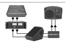
Add powered monitors on stage The SP-2SX lets you take the speaker output from a wedge monitor and feed it to a set of powered monitors for the drummer or side fills. Simply connect into the SP-2SX, set the power level to suit, and it will deliver a distortion-free line level signal.
