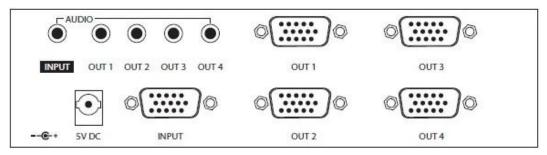
The Intelix VGA2-DA4 is a one input by four output VGA video and stereo audio distribution amplifier. The VGA2-DA4 supports resolutions up to 2560x1600 and 20Hz to 20kHz stereo audio up to 300 feet (91 meters).
