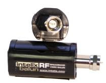
The Intelix RF-F balun passively transmits broadband (RF) video over unshielded twisted pair cabling, such as Cat 5 or Cat 5e. Used in pairs, the RF-f transmits video up to 330 feet, providing a low-cost versatile cabling solution which uses a building's existing structured cabling system.
