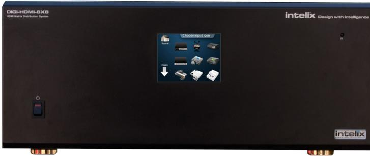
Why settle for mediocrity? The Intelix DIGI-HD-8X8 combines a professional-grade HDMI matrix with Intelix's industry-leading extenders. Each system provides eight HDMI inputs, eight HDMI outputs, and eight twisted pair outputs. Plus, a built-in touch screen delivers front panel source selection and matrix routing with ease. Third-party control systems integrate seamlessly via RS232, Ethernet or IR.
