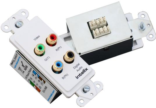
The Intelix AVO-V3AD-WP110 wallplate balun transmits one component video and one digital audio signal over standard unshielded twisted pair cabling, such as Cat 5 or Cat 6. Used in pairs or with a compatible Intelix balun, the AVO-V3AD-WP110 transmits signals up to 500 feet and is ideal for corporate A/V, churches, schools, auditoriums, and almost any other situation involving audio/video distribution.
