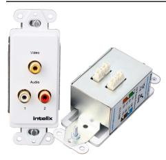
The Intelix AVO-V1A2-WP110 wallplate balun transmits one composite video and one stereo analog audio signal over standard unshielded twisted pair cabling, such as Cat 5 or Cat 6. Used in pairs or with a compatible Intelix balun, the AVO-V1A2-WP110 transmits signals up to 2,200 feet and is ideal for corporate A/V, churches, schools, auditoriums, and almost any other situation involving audio/video distribution.
