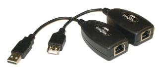
The Intelix AVO-USB extender set transmits low and full speed USB signals over twisted pair cabling. The set extends low speed USB 1.0 and 2.0 signals up to 330 feet, and full speed USB 1.0 and 2.0 signals up to 100 feet. Convenient connector dongles allow direct connection to the host and client devices, facilitating a clean, low-profile installation.
