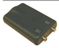
The Intelix AVO-A2 balun transmits two mono or a single stereo analog audio signal via standard structured cabling, such as Cat 5. Used in pairs, the AVO-A2 transmits analog audio in either direction up to 2,500 feet and is ideal for corporate A/V, churches, schools, auditoriums, and almost any other situation involving audio distribution.
