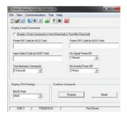
Intelix ASW-WP Display Control software provides seamless control of the connected display or projector. Route power on/ off commands and input select commands via RS232, and preset power down commands based on inactivity.
