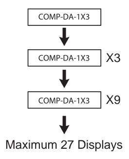
Maximum recommended distance of component cabling between each 1:3 Component Audio DA or display (1080p) is 50 ft. Maximum number of displays that are supported in a large 1:3 Component Audio DA system is 27.
