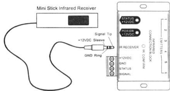
**IR Receiver In:** This is a three terminal 1/8" plug that is common to many of the free standing IR receivers. This will connect the power, ground and signal. Signal is Tip, ground is the ring and power is the sleeve.
