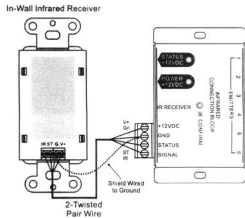
Remote IR receivers may be connected to the detachable connector labeled +12VDC, GND, STATUS, and SIGNAL.
