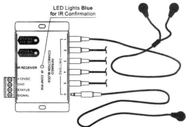
**Emitter Outputs:** Connect up to 6 emitters (to the emitter jacks labeled 1-6. Place the emitters on the source equipment.
