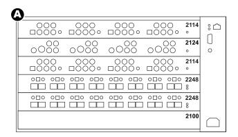
Example A incorporates the 2124 source card which offers SD inputs, scaled to Y Pb Pr. Useful for adding security camera feeds and/or legacy sources into the HD distribution system.
