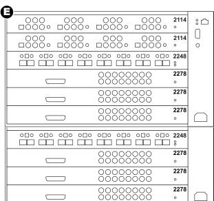
Example E represents the maximum number of zones (64 zones) using the expanded card cage. Video and audio zone cards can be mixed in any order.
