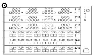
Example D shows the maximum number of video sources\* (12) with the maximum video zones (24) in a single card cage.
