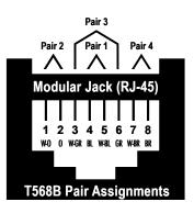
WARNING: continuity testing is not adequate; the twisted pairs must be placed in precise order in the connector, or damage to the equipment may occur.
