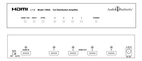
The 1394A has a single HDMI input and four HDMI outputs. The 1398A has eight outputs. The Power LED indicates that the unit is receiving power.
