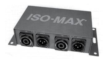
The Iso•Max SP-2SX is a two channel speaker to line level converter that lets you convert the high power signal from an audio amplifier output to a +4 dB (nominal) balanced line level for further processing or signal distribution.
