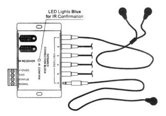
**Emitter Outputs:** Connect up to 6 emitters (to the emitter jacks labeled 1-6. Place the emitters on the source equipment.
