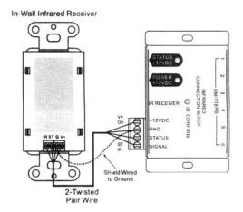
Remote IR receivers may be connected to the detachable connector labeled +I2VDC, GND, STATUS, and SIGNAL.
